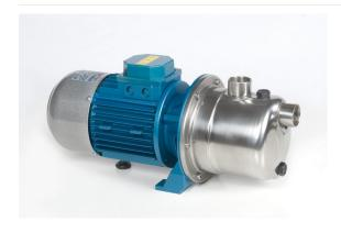
Self-priming centrifugal electric pumps of jet type, suitable for pumping and pressurizing clean water up to 60 ° C. They are equipped with an ejector that guarantees high suction and self-priming capacity and operation even in the presence of gas dissolved in the liquid. The ECC JET series is made of AISI 304 stainless steel and technopolymer, it is provided with a 12V or 24V DC motor.
