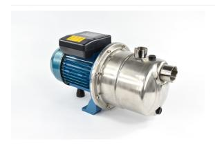
Self-priming centrifugal electric pumps of jet type, suitable for pumping and pressurizing clean water up to 60 ° C. They are equipped with an ejector that guarantees high suction and self-priming capacity and operation even in the presence of gas dissolved in the liquid. The JIM series is made of AISI 304 stainless steel and technopolymer, it is provided with a single-phase asynchronous motor.
