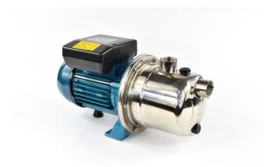
Self-priming centrifugal electric pumps of jet type, suitable for pumping and pressurizing clean water up to 60 ° C. They are equipped with an ejector that guarantees high suction and self-priming capacity and operation even in the presence of gas dissolved in the liquid. The JIM series is made of AISI 304 stainless steel and technopolymer, it is provided with a single-phase asynchronous motor.
