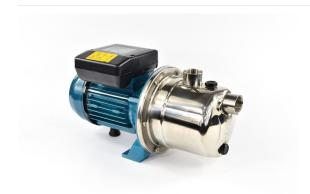
Self-priming centrifugal electric pumps of jet type, suitable for pumping and pressurizing clean water up to 60 ° C. They are equipped with an ejector that guarantees high suction and self-priming capacity and operation even in the presence of gas dissolved in the liquid. The JIM series is made of AISI 304 stainless steel and technopolymer, it is provided with a single-phase asynchronous motor.
