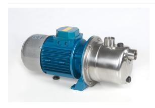
Self-priming centrifugal electric pumps of jet type, suitable for pumping and pressurizing clean water up to 60 ° C. They are equipped with an ejector that guarantees high suction and self-priming capacity and operation even in the presence of gas dissolved in the liquid. The ECC JET series is made of AISI 304 stainless steel and technopolymer, it is provided with a 12V or 24V DC motor.
