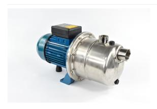
Self-priming centrifugal electric pumps of jet type, suitable for pumping and pressurizing clean and drinking water up to 60  $^{\circ}$  C. They are equipped with an ejector that guarantees high suction and self-priming capacity and operation even in the presence of gas dissolved in the liquid. The JIM series is made of AISI 304 stainless steel and technopolymer, it is provided with a three-phase asynchronous motor.
