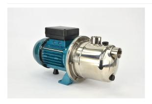
Self-priming centrifugal electric pumps of jet type, suitable for pumping and pressurizing clean and drinking water up to 60  $^{\circ}$  C. They are equipped with an ejector that guarantees high suction and self-priming capacity and operation even in the presence of gas dissolved in the liquid. The JIM series is made of AISI 304 stainless steel and technopolymer, it is provided with a three-phase asynchronous motor.
