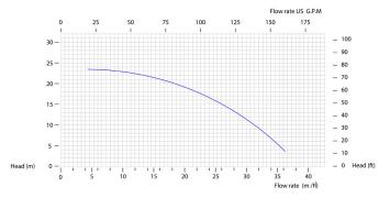
The curves and performance values refer to pumps with free delivery outlet with water at 20 °C, and two poles motor 50 Hz. These data may vary according to the construction materials and hydraulic conditions.
